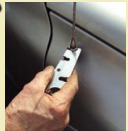
The Antenna Wrench II being used on a Dodge truck with raised hood.
